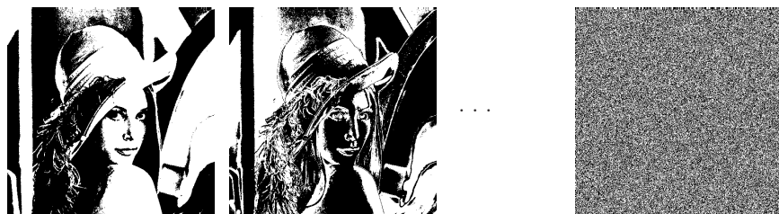
Fig. 6. Most significant, second significant and least significant bit-plane for 512 \times 512 grayscale image lena
